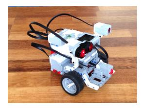
I thought a good first step in learning about Lego Mindstorms EV3 was to build a Tribot and have it drive around a square 1m on edge. There is a plethora of information about EV3. Do a Google search on "build EV3 Tribot" or "EV3 drive in a square". The number of sites identified is overwhelming and it's difficult choosing where to start. The Art of Lego Mindstorms EV3
