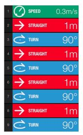
Writing the code to direct the Parrot drone to drive in a square is straightforward. The Parrot iPad app has the macro commands for "straight" and "turn" as shown in the code to the left. The only shortcoming is that "loops" are not available so the commands to drive straight 1m and turn right 90 degrees have to be repeated 4 times.
